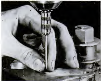
If the pointer wiggles, the work is off center
